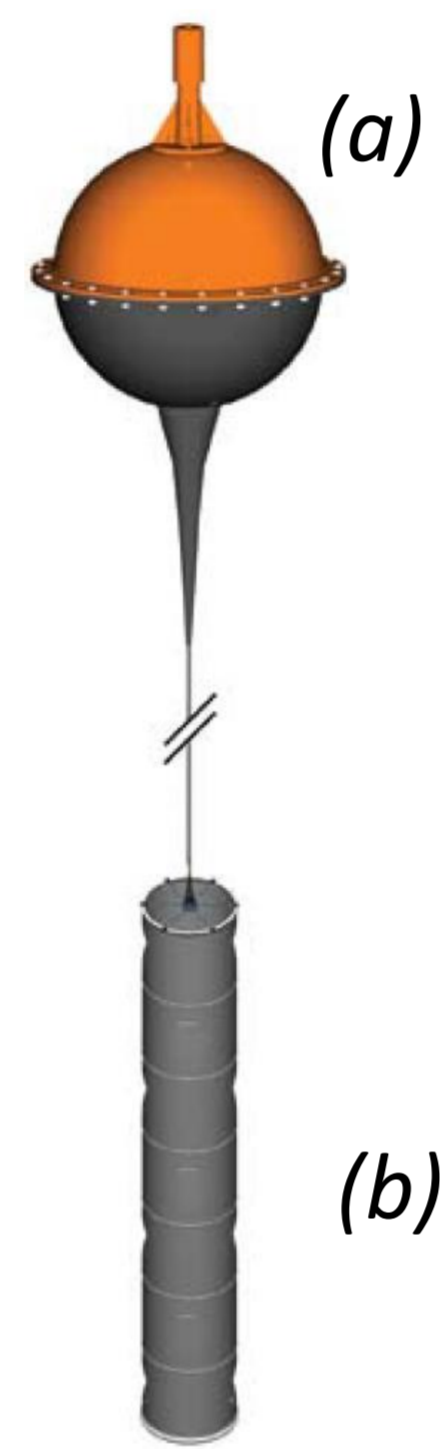
Figure 2. Left: Drifter right after deployment with drogue still folded. Right: Drifter (a) with unfolded drogue (b).
